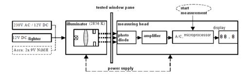
Block diagram of the device
